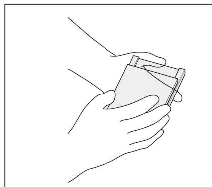
2. Slide the two plates into the Casting Frame, keeping the Short Plate facing front. Insure both plates are flush at the bottom on a level surface.
