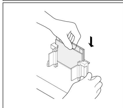
3. Lock the pressure cams to secure the glass plates.
