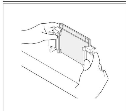
4. Engage the spring loaded lever and place the gel cassette assembly on the gray casting stand gasket. Insure the horizontal ribs on the back of the Casting Frame are flush against the face of the Casting Stand and the glass plates are perpendicular to the level surface. The lever pushes the Spacer Plate down against the gray rubber gaskets.
