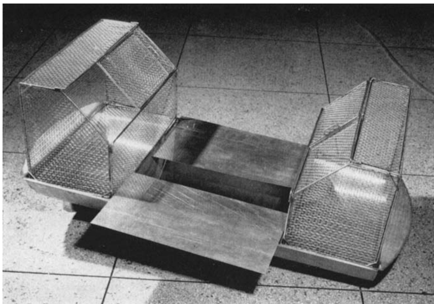
FIGURE 15. Chicken pens and floor for RSU-300 isolator. The center compartment is for storage of supplies, and the wire cages set over compartments to collect waste. These pens also can be used for guinea pigs and rabbits.
